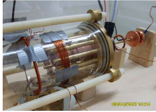
Figure 2. b) The vacuum chamber with electrodes inside, field coils and spark gap.
