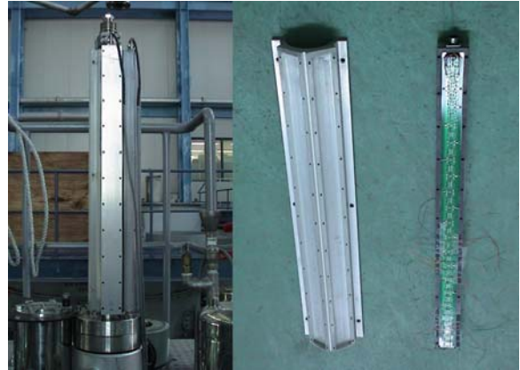
Fig 5 Photograph of arrangement of the reed switches
