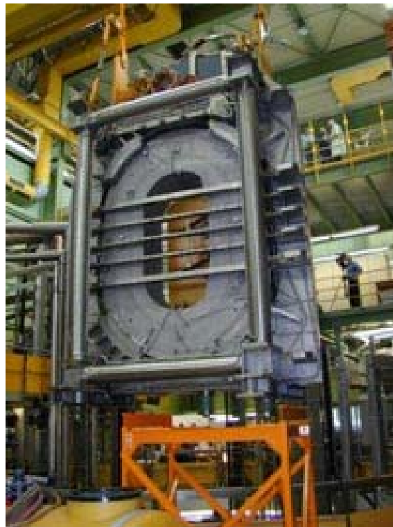
Figure 8 – View of prototype of the ITER toroidal magnetic field coil
